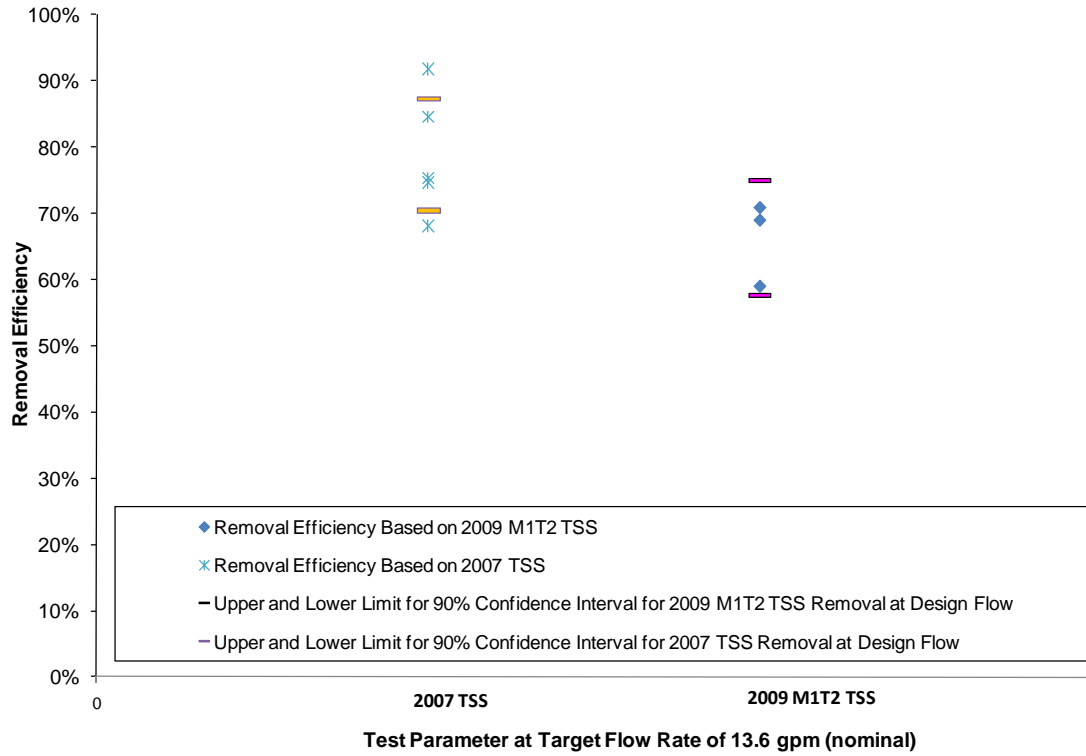
Figure 13. M1T2 performance results compared to 2007 Perk Filter™ results at 13.6 gpm.
